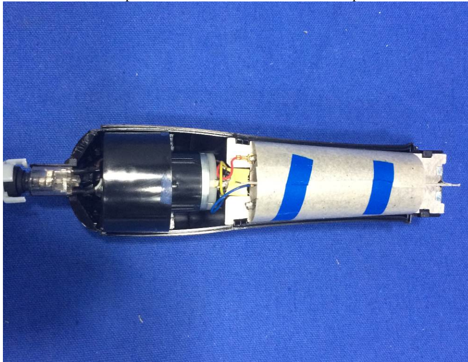
Description: Internal view of HT-8600 with X2 capacitor
