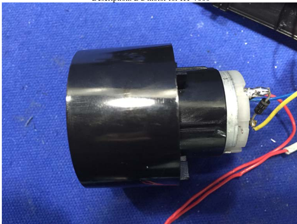
Description: DC motor for HT-7000
